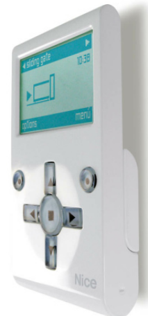
O-View programmer is used by the installer to advance features and fine tune motor functions.
