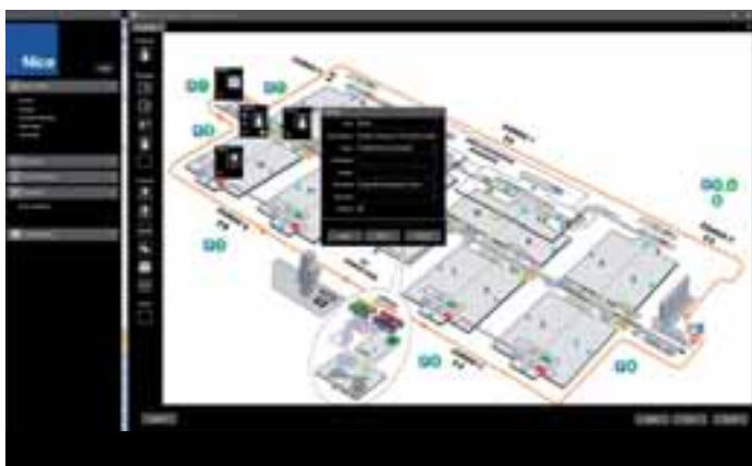
Basic level plant configuration mode allowing generation of the list of materials needed for realisation of the car park.
